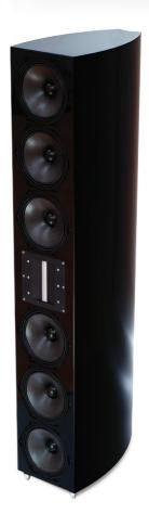
The Raven R3.2MMX ribbon covers all midrange and treble above 800 Hz. This is the most critical range for imaging and intelligibility. Covering this entire frequency range with a single ribbon is important to a coherent presentation. The special MMX ribbon material is 6 times stronger than common aluminum so it is very robust and can play much louder without distortion.
